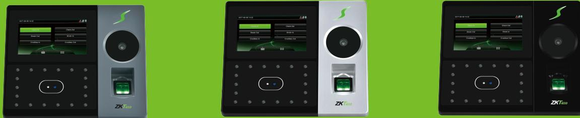
PFace202 multi-biometric time & attendance and access control terminal supports up to 600 palm templates, 1,200 face templates, 2,000 fingerprint templates and 10,000 cards (optional).
